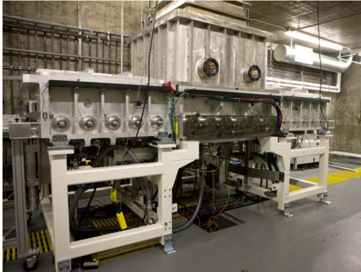
High-Energy Proton Implanter Prototype (up to 150um)
