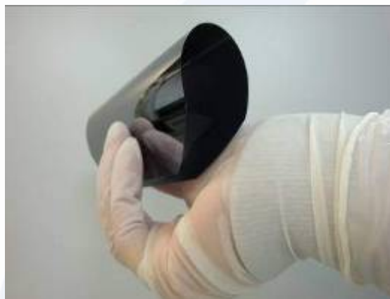
20um Silicon Wafer (2009)
