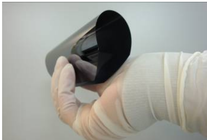
125mm x 125mm – First ever kerf-free 20um Mono c-Si Solar PV Foil
